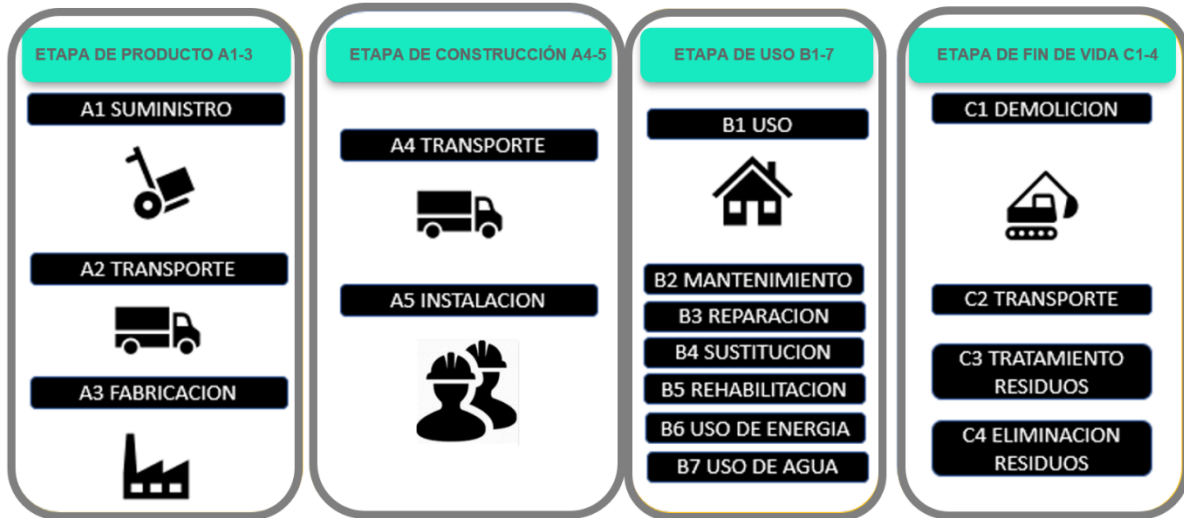
Figure 2: Stages of the life cycle of a product according to the analysis "from the cradle to the grave".
